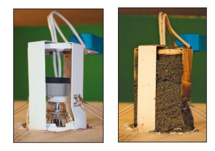
This patented and registered design, incorporates a unique intumescent reaction allowing a totally new concept as a cage constructed luminaire.
